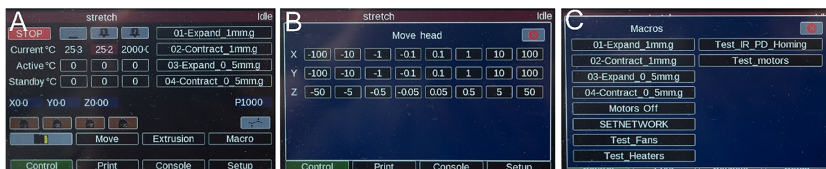
Fig. 21. Images of PanelDue control screens. (A) Main screen (B) Move screen (C) Macro Screen.
