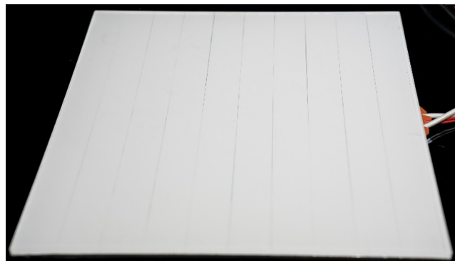
Fig. 3. Picture of the assembled heated bed plate.
